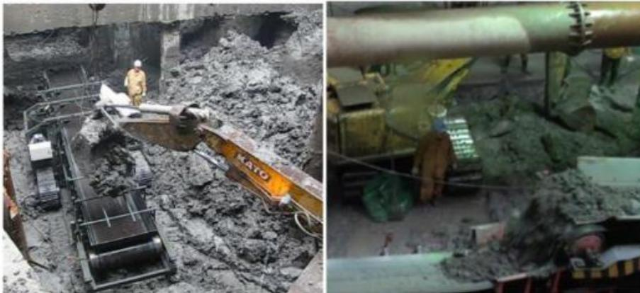
**Figure 7.** Field tests of the track-type belt conveyor.
