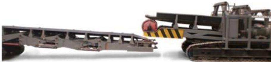
Figure 5. Photograph of two overlapped TTBCs.
